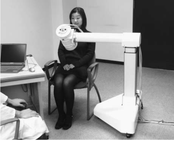
Fig. 15. Open-SQUID MCG detection system. A patient is sitting on a chair and need not lie down
