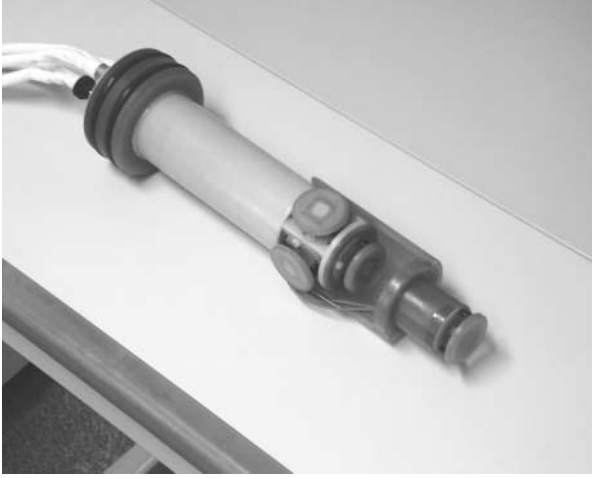
Fig. 13. Experimental set-up of four magnetometers in a specially designed susceptor
