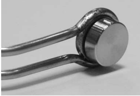
Fig. 7. Aurora PLD with the magnet at the shadow mask position
